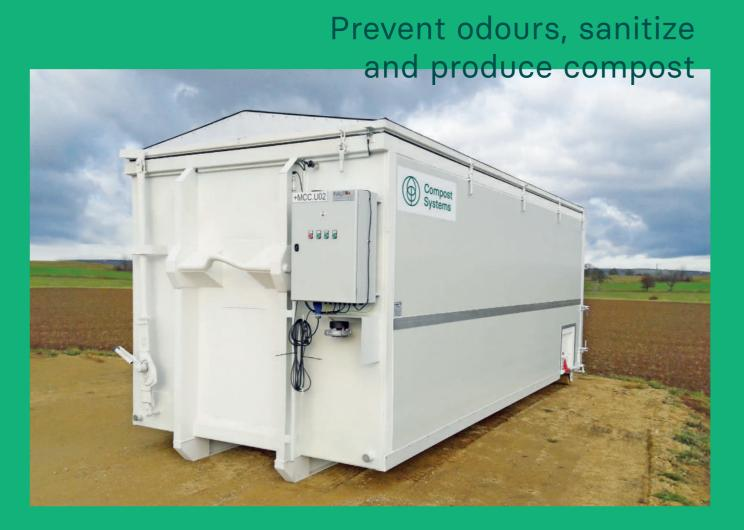
The lid is equipped with a semi-permeable membrane, which allows odour-free operation when the lid is closed. The lid has an all-round seal and is secured by means of tension locks. The rotary and pendulum flap at the rear is designed to be watertight and is also secured with tension locks.
