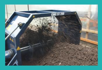
The scope of supply of the CMC ST 200 kit includes the entire steel structure (incl. steel tubes and cut sheet metal), as well as all components, such as gearbox, hydraulic cylinder and hydraulic hosing, tires, axle and PTO shaft. The rotor is fully assembled, but only tack welded. The buyer must finish welding the rotor. The kit is supplied with comprehensive assembly instructions.
