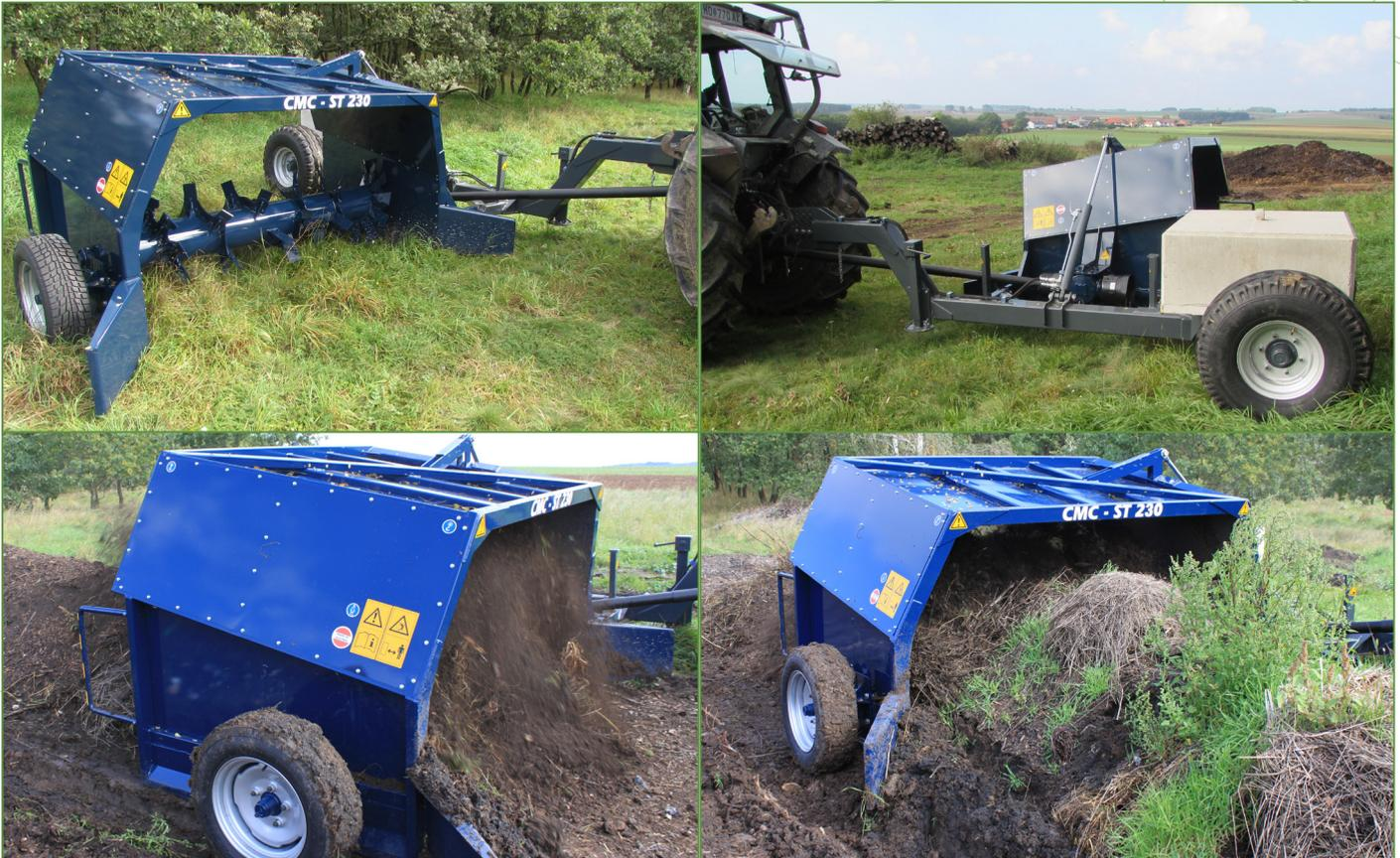
The new **CMC ST 230** offers high performance with compact design. The machine creates perfect mixing and ventilation results for tractors of minimum 30 hp. With a net tunnel opening of 2.3 m the machine can turn compost windrows up to a width of 2.6 m. Built on a trailer, in the proven system, the machine
