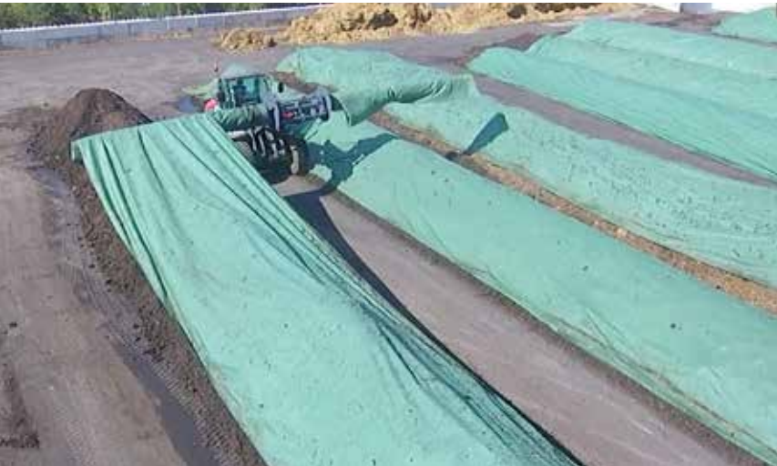
Compost protection fleece in use in an Austrian facility
