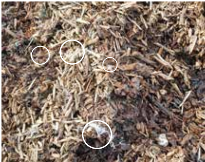
Plastic fibres distributed throughout the material
