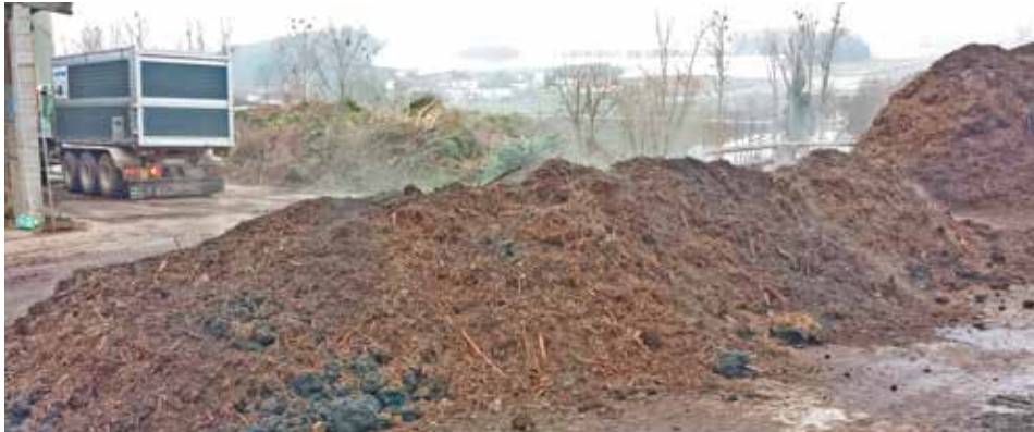
Quality sewage sludge was mixed with bulking material and processed into high-value quality compost of Class A.
