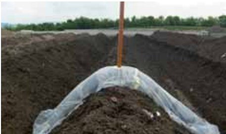
To secure comparable results under all weather conditions, a special testing tool was built, that provides same conditions for all sampled windrows.
