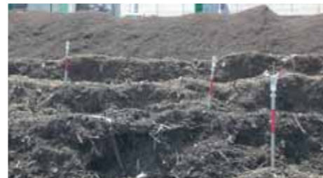
COMPOtemp remote probes in use
