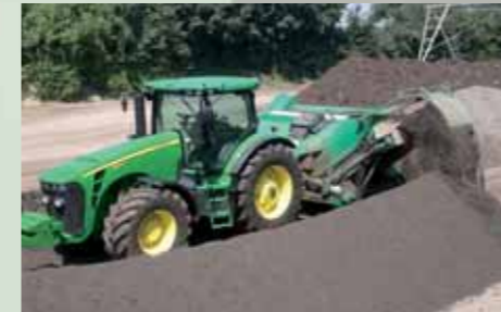
The TracTurn easily cuts windrows up to 2.3 m height apart.
