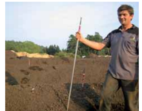
Compost plant Huemer (A) with temperature monitoring of the main compost platform
