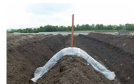
Collection of the odour emissions over the entire windrow width
