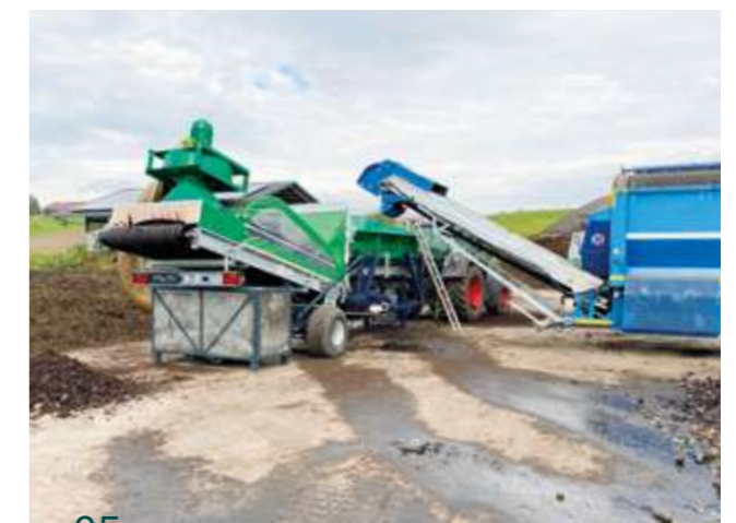
03 Stationary screen with air separator and large hopper
