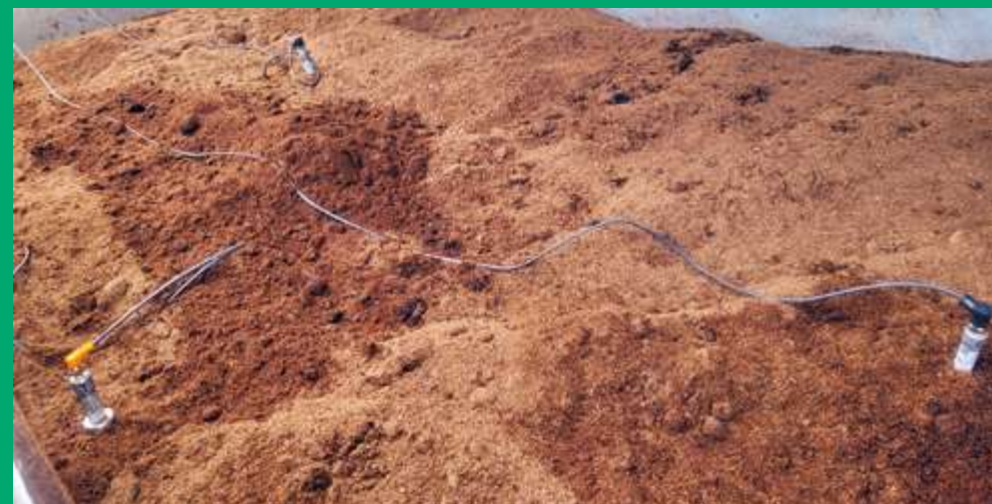
Sensors for controlled aeration and sanitization verification.
