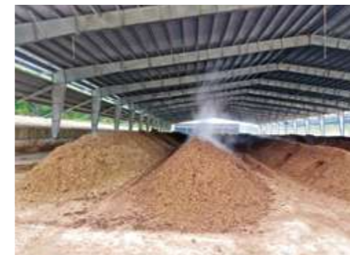
Here, pressed slurry, digestate and other agricultural waste are processed into a high-quality fertiliser.
