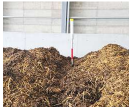
Here, digestate is transformed together with other waste and straw into a high-quality compost fertiliser within 6–8 weeks.
