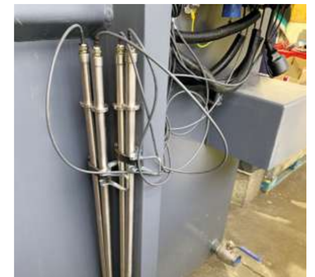
Four temperature probes connected simultaneously.
