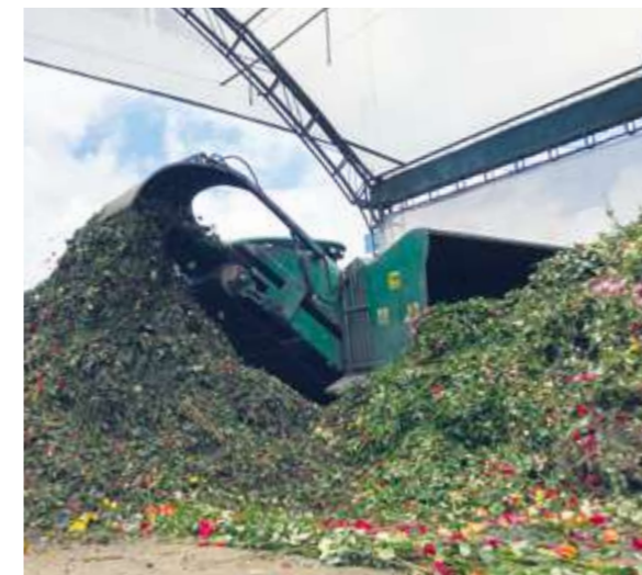
In addition to the aeration system, the TracTurn compost turner from Compost Systems is also employed at the Control Ambiental plant – here for the composting of flowers.
