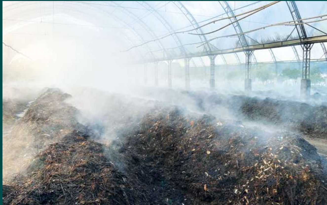
Composting windrows under controlled conditions using forced aeration technology supplied by Compost Systems.
