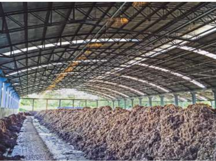
In the palm oil industry, around 3 tonnes of liquid waste are generated for every tonne of solid waste. With optimised process control, the water can be evaporated within the process itself. What remains are the nutrients, carbon and minerals in the form of biofertiliser – or, as we call it, high-quality compost!
