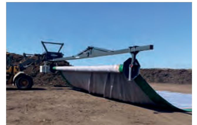
Fleece and membrane winders help with the handling of compost covers.
