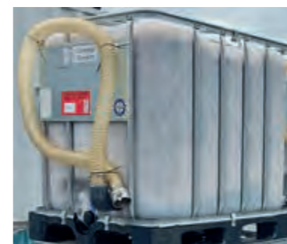
Biofilter of a CSC-Container.
