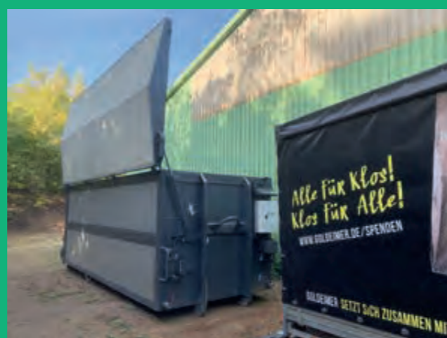
CSC-Container for the hygienisation of the material.
