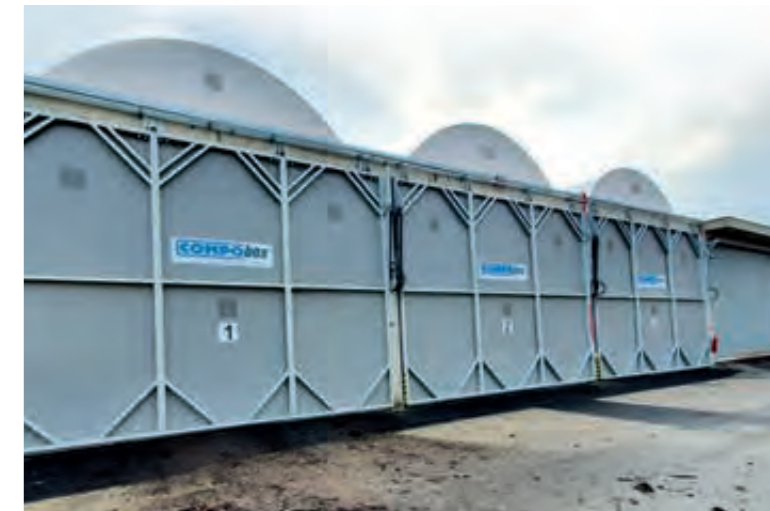
Composting in a closed system (CSC or box) and subsequent maturation.
