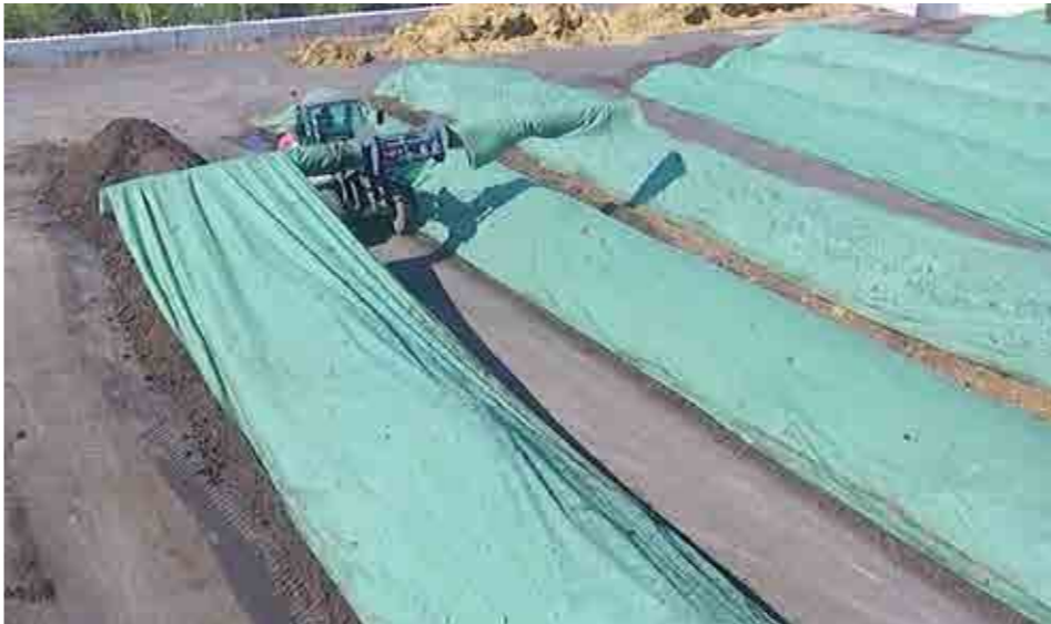
Compost fleece used at an Austrian facility
