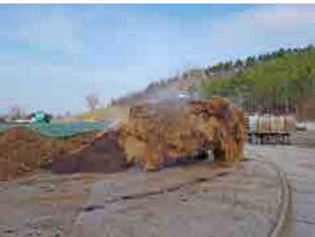
The installed aeration makes it possible to limit the turning to just once a week.
