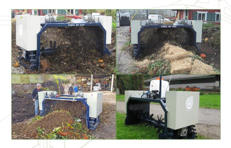
The CMC SF 200 is a self propelled electric drive turning machine ideally suited for small plants. It has proven to be an excellent machine with an ideal mixing ability, simple handling by a manual control unit. Space requirements are kept to a minimum and
